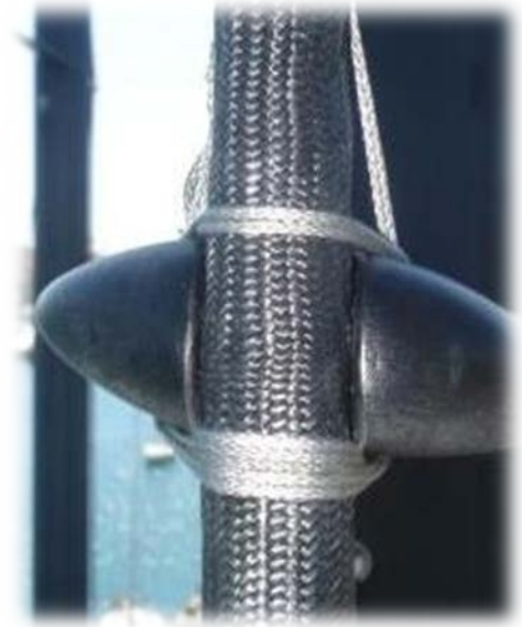
Figure 3a & 3b: EC6+ top spreader tip lashing
