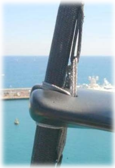
Figure 2: EC6+ top spreader tip lashing
