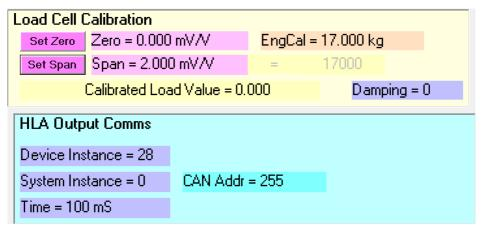
Make sure the "Device Instance" matches the value for the load cell position (from instrument setup).
