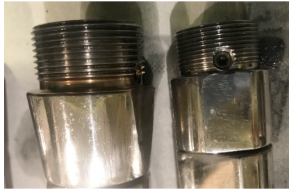
Adjusters studs without damage or wear on threads
