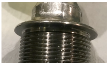
Noses of D1 and CP-D2 without damage or wear
