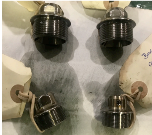
Noses of D1 and CP-D2 without damage or wear
