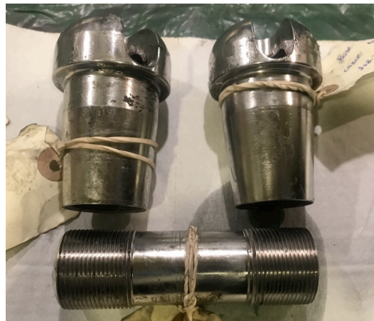
CR-D3 tangs and throughmast bar. In a good serviceable condition
