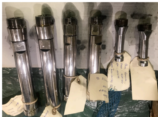
V1, D1 and CR-D2 adjusters. No damage was detected on the parts
