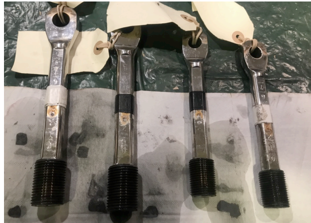
Eye studs, V1 and D1. No damage detected on threads and eyes
